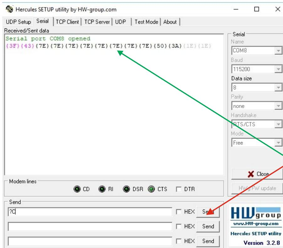
Push this button, in this mode the string "?C" is transmitted (request of configuration)
