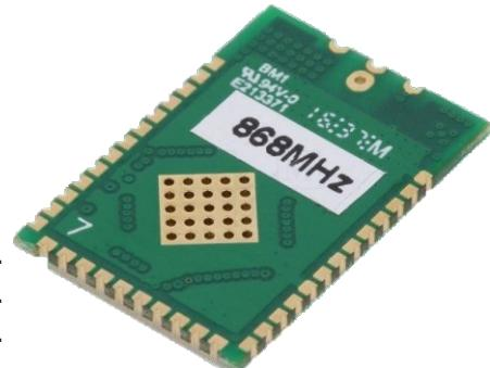
The RF modem is very simple to use and provides a wireless RS232 link with a RF data rate of up to 50kbps. The transceivers have the functions of a complete radio modem and simply require CMOS/TTL data at the transmit input and the corresponding transceiver(s) output the same data. Preamble and CRC are automatically generated and added to the RF transmission.
