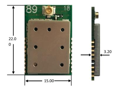
Unit: mm Tolerance: 0.2mm
