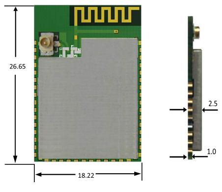
Unit: mm Tolerance: 0.2mm
